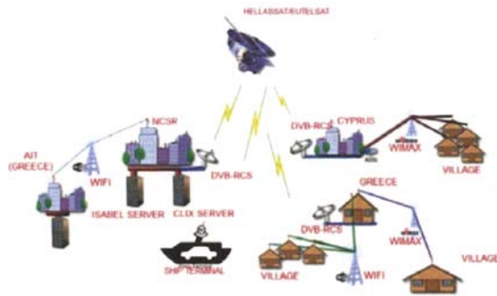
Figure 1. Base 2 Generic Satellite and Wireless Network Architecture
