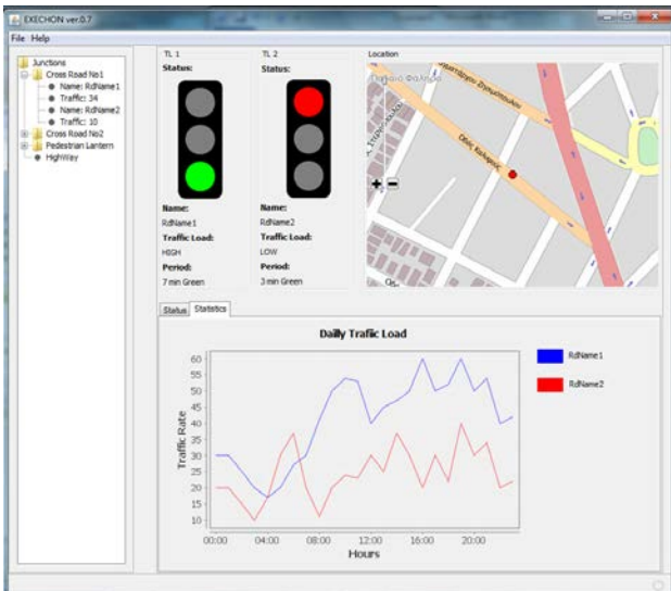
Fig. 6: Graphical Representation of the sensed data at the city traffic management center (traffic load evolution with time)
